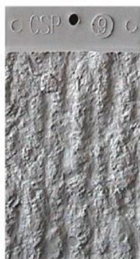
CSP-9: Heavy Scarification
