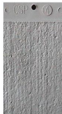
CSP-4: Light Scarification
