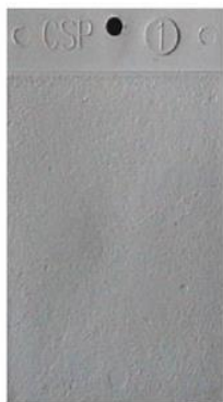
CSP-1: Acid Etched*
