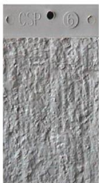
CSP-6: Medium Scarification
