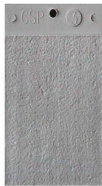
CSP-3: Light Shot Blast
