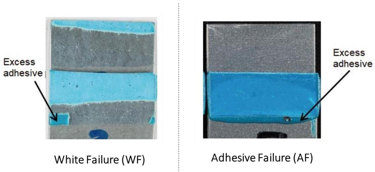
**Figure 24** Difference between white failure (WF) and adhesive failure (AF) as in Technical Code DVS 3302 [8].
