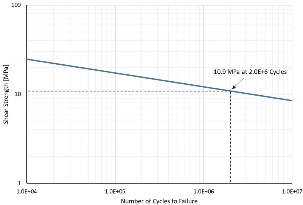
**Figure 19** Exemplary fatigue curve for SikaPower® epoxy adhesive.
