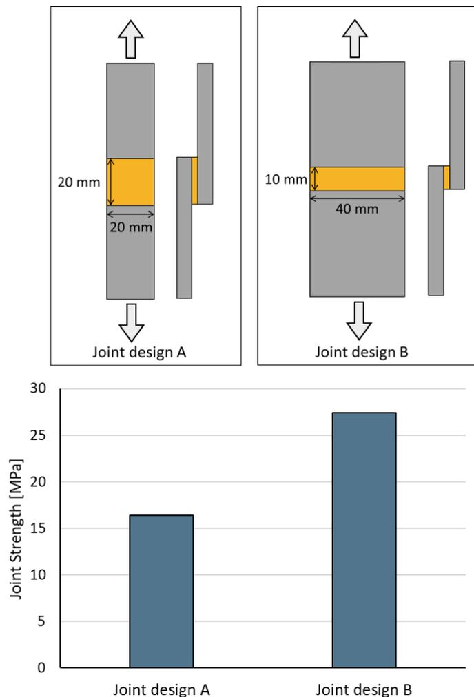
**Figure 11** Strength comparison of joints bonded with the same rigid SikaPower® adhesive: the two joints have equal areas but different overlap length and width, resulting in different final strength.
