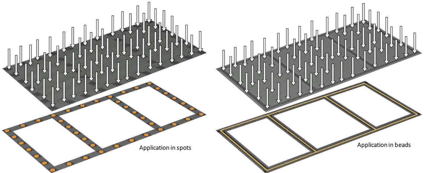
**Figure 8 (A)** Stress analysis of a stiffening frame bonding with spot application (left picture) and bead application (right picture): forces and joint configurations.
