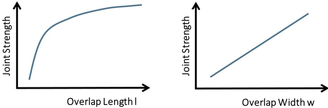
**Figure 10** Effects of overlap length and width on joint strength in single lap shear.
