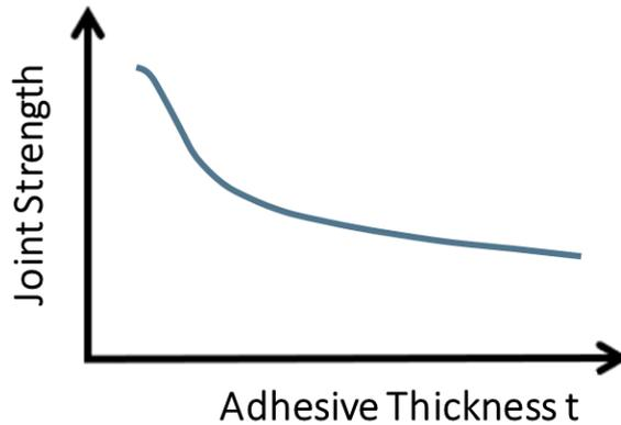
**Figure 12** Effects of adhesive thickness on joint strength.
