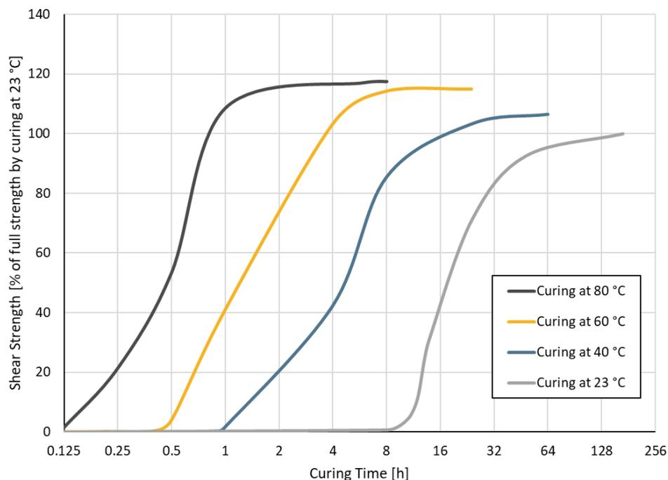
Figure 28 Exemplary strength build-up of 2C epoxy at various curing temperatures.
