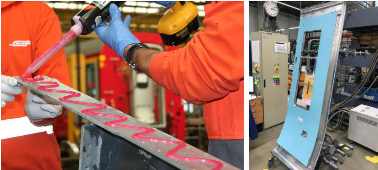
**Figure 18** Railway vehicle door bonding with a SikaPower® adhesive.
