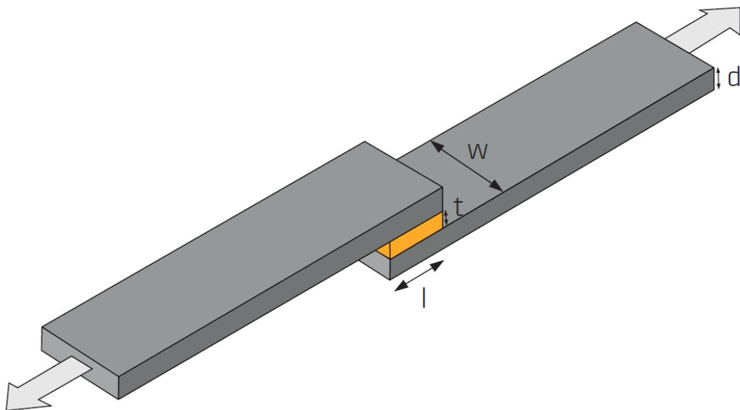
**Figure 9** Single lap joint geometry.
