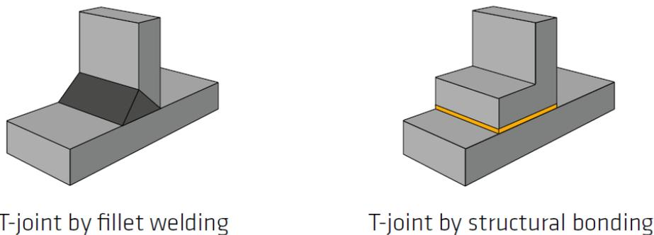
**Figure 1** T-joint design examples for welding and bonding.
