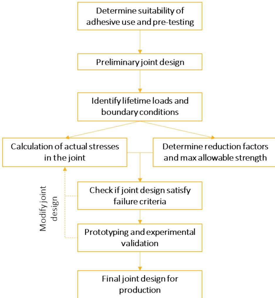
**Figure 21** Procedure to design bonded joints.
