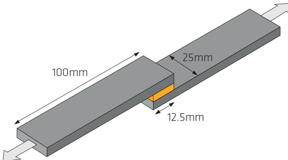
Figure 23 Specimen size for lap-shear tests.
