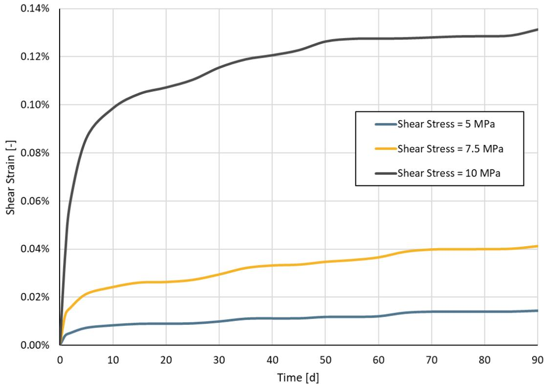
**Figure 26** Exemplary creep curves for SikaPower® epoxy adhesive.
