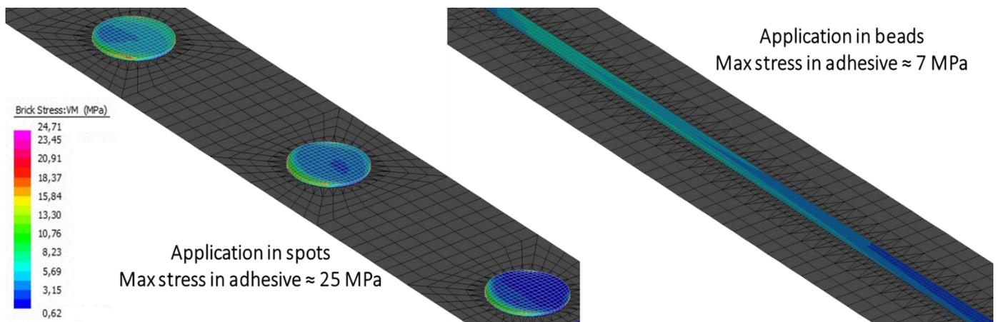
**Figure 8 (C)** Stress analysis of a stiffening frame bonding with spot application (left picture) and bead application (right picture): stress distribution in the adhesive.
