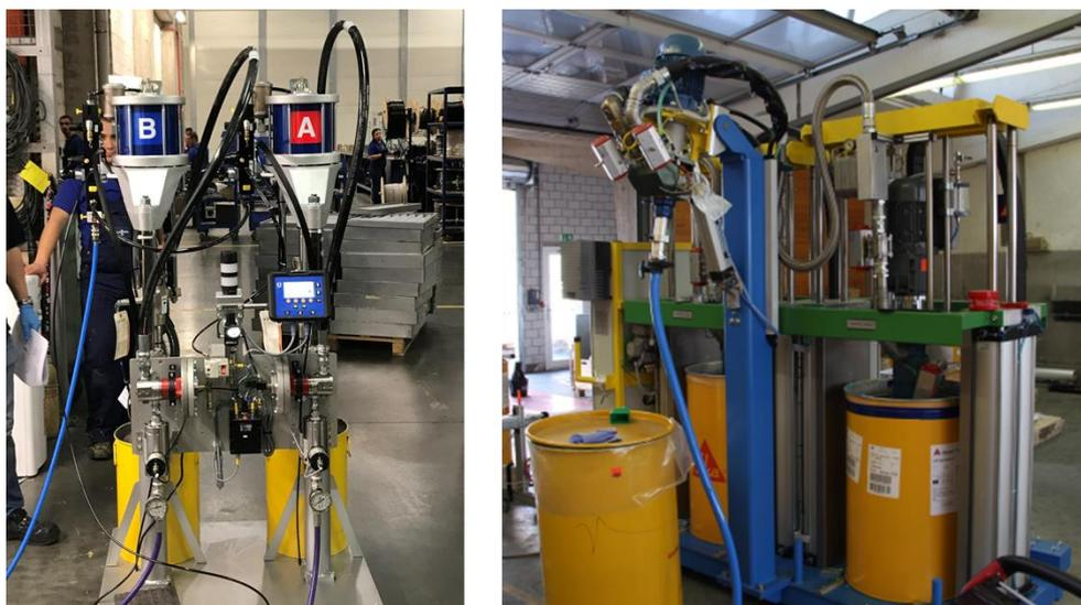
**Figure 35** Dispensing equipment for two-component adhesives out of pails (left) and drums (right).
