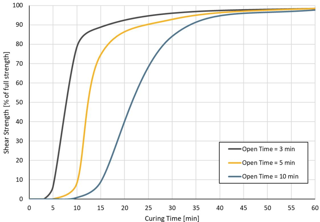
Figure 32 Exemplary strength build-up of 2C acrylic-based adhesives.
