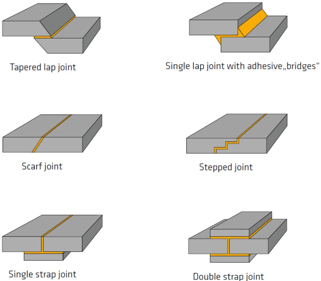
**Figure 6** Improved configurations for simple lap joints.
