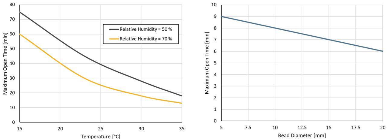
**Figure 34** Exemplary open time dependency on humidity (for a slow curing polyurethane) and bead size (for a fast curing polyurethane).
