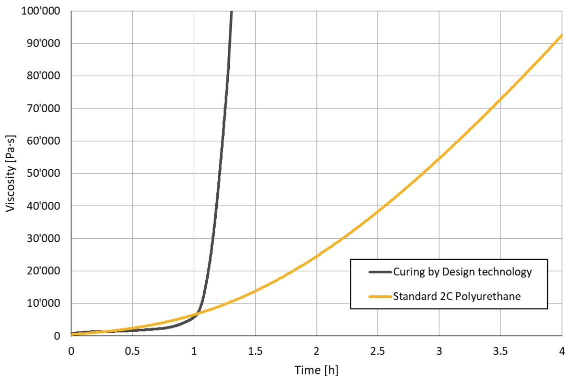
**Figure 31** Comparison of curing behavior of Curing by Design technology and a standard 2C polyurethane with same working time.
