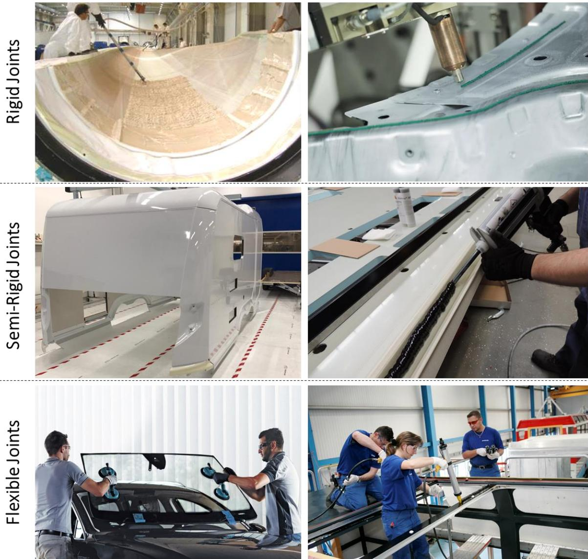
**Figure 14** Exemplary industrial applications of bonded joints: rigid (wind turbine blade and metal chassis bonding), semi-rigid (caravan and bus modular bonding) and flexible (windshield and panel bonding) joints.
