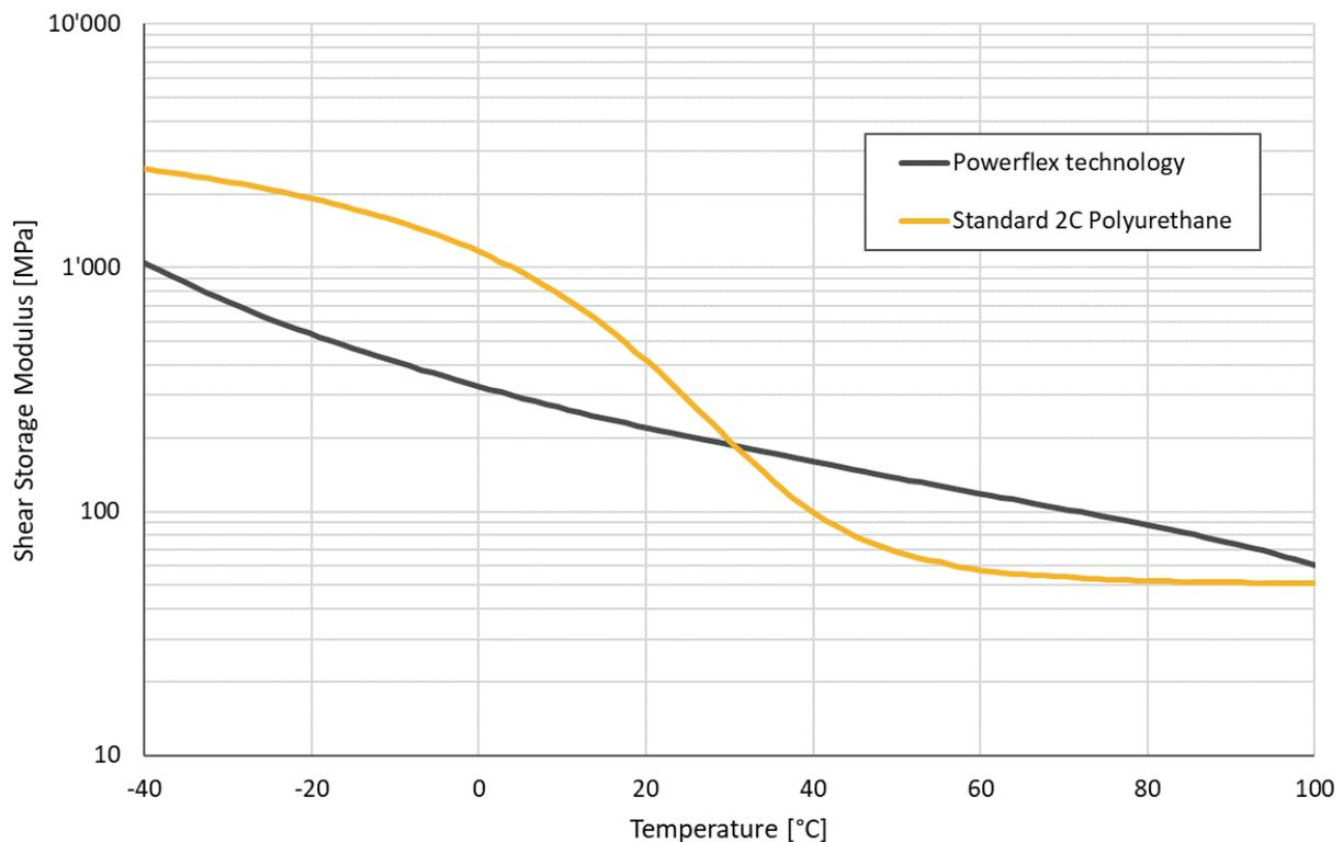
**Figure 30** Comparison of shear modulus of Powerflex technology and a standard 2C polyurethane from DMA tests.
