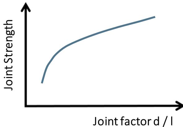
**Figure 15** Joint strength as a function of the joint factor (substrates thickness to overlap length ratio).
