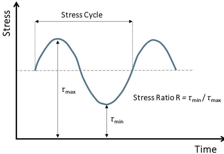
Figure 27 Cyclic stress in fatigue tests.
