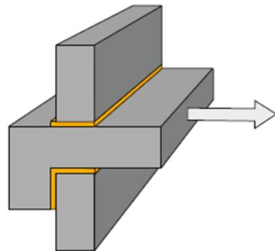
Figure 4 (C) Best practices for bonded joint design.
