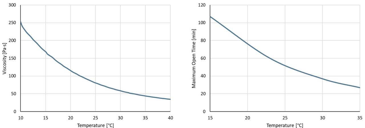
**Figure 33** Exemplary viscosity and open time as function of application temperature.
