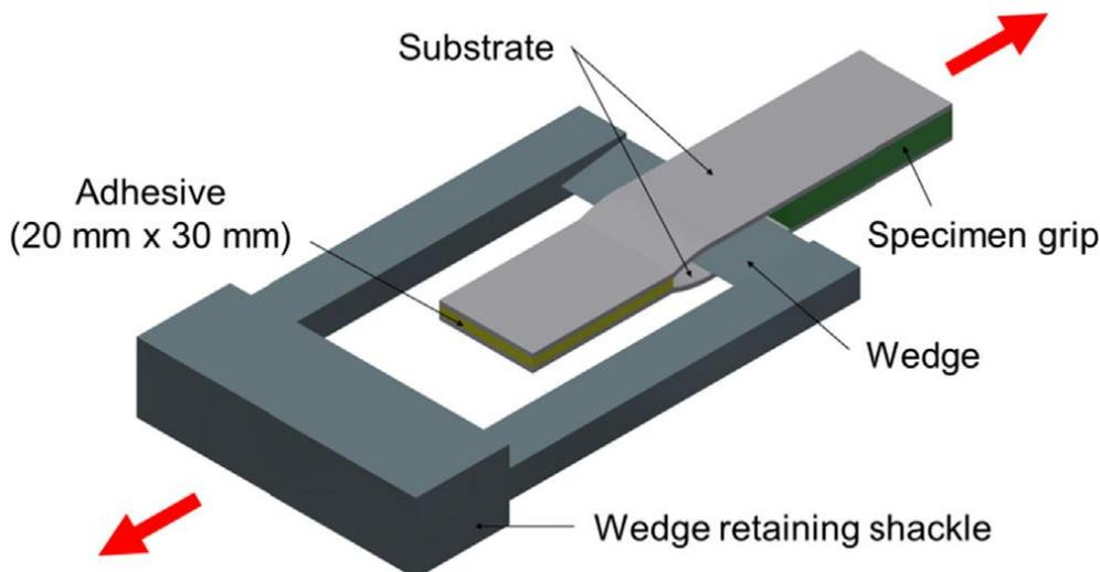
Figure 25 Impact wedge peel test set-up.
