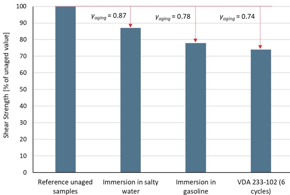
Figure 17 Exemplary reduction factors for environmental aging of a SikaPower® adhesive.
