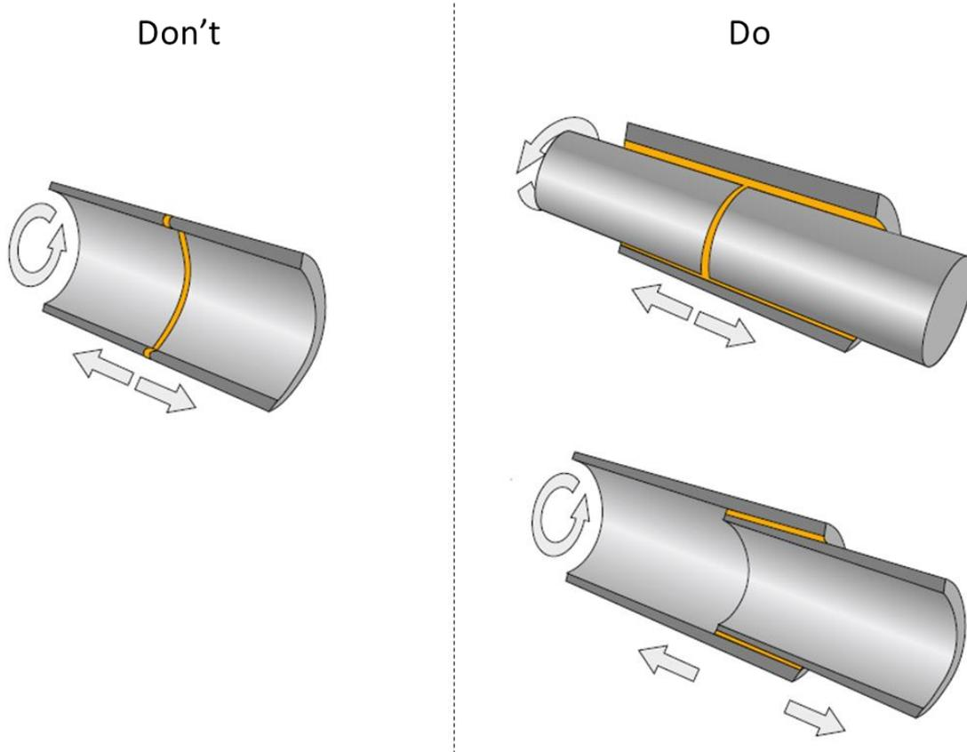
Figure 4 (I) Best practices for bonded joint design.
