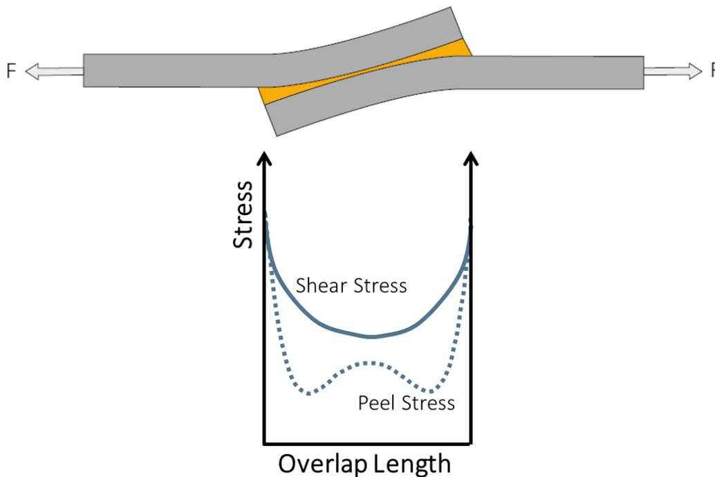
Figure 5 Bending and stress peaks in single lap joints.
