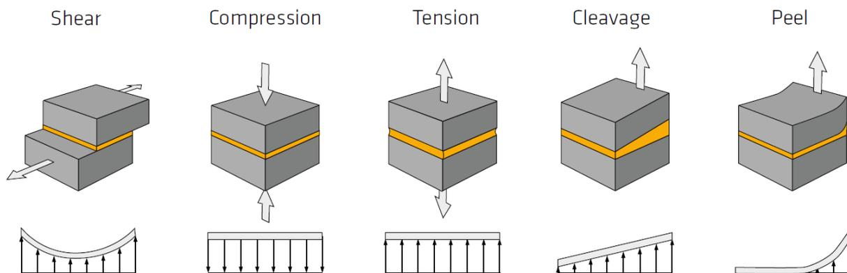
**Figure 3** Fundamental types of stresses in bonded joints.
