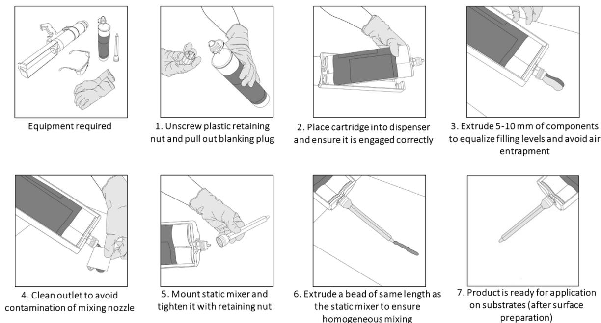
**Figure 36** Instruction for application of 2C adhesives out of cartridges.
