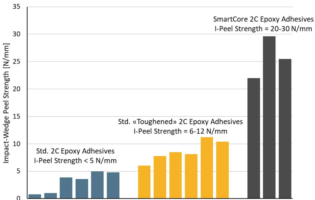
**Figure 29** Comparison of impact-wedge peel strength of standard, toughened and SmartCore 2C epoxies.
