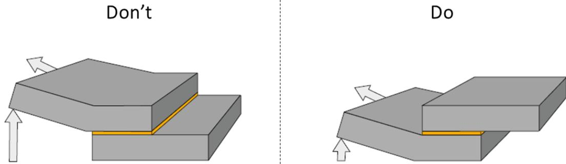
**Figure 4 (D)** Best practices for bonded joint design.
