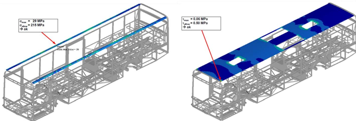
**Figure 20** Stress analysis and failure criteria checks for bus roof bonding application [7].
