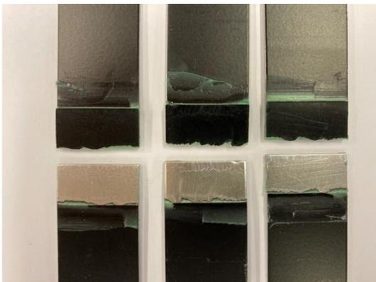
Coating rupture in powder coated metals
