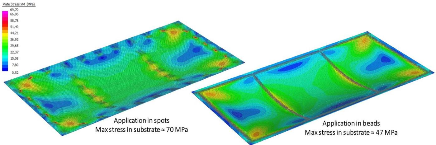
**Figure 8 (B)** Stress analysis of a stiffening frame bonding with spot application (left picture) and bead application (right picture): deformation and stress in the substrate plate.
