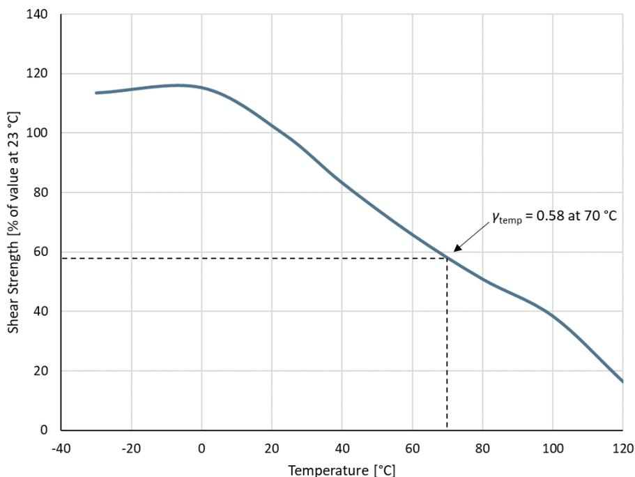
**Figure 16** Exemplary temperature dependency of the adhesive strength.
