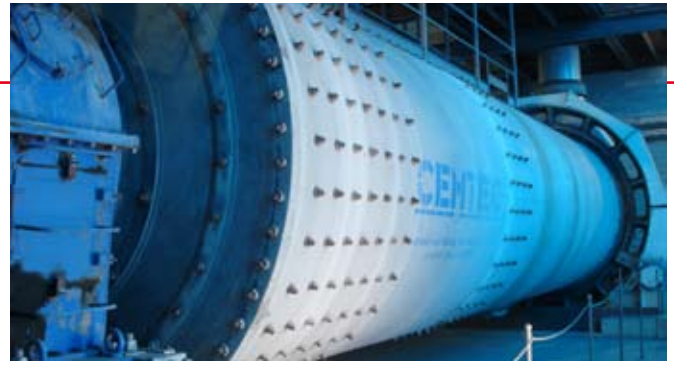
The cement mill is the last production step in cement manufacturing
