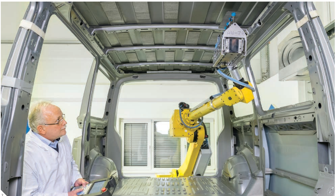
1 Expanded SikaBaffle® in steel cavity 2 Automated application of SikaDamp®
