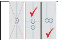
Welds at transverse joints. By proper arrangement of Sarnafil® AT, all seams can be reduced to straight welded seams and transverse joint (T-joint). Cross joints are to be avoided.
