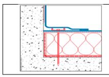
Sarnabar® to be applied all along the roofing perimeter.
