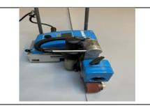
Membrane overlaps are welded by using a hot-air welding machine.
