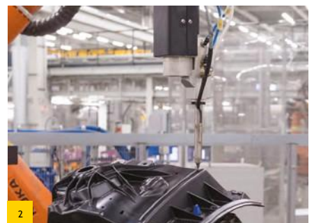
SikaPower® application at shock tower
