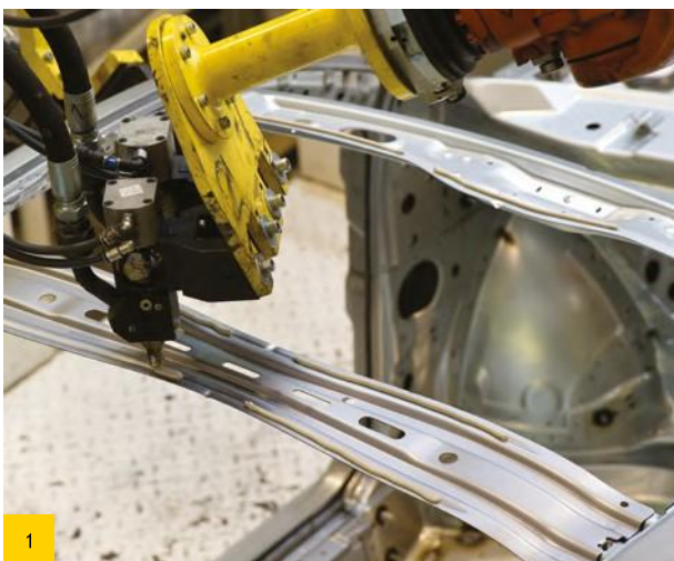
1 Roof cross member anti-flutter application 2 Finished roof application to the body frame
