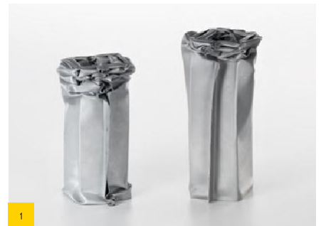
Crash beams without (left) and with SikaPower® (right)
