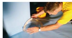
*Vacuum testing of a detail*
